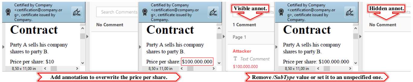
Figure 5. A certified document. The Price per share was manipulated by a FreeText annotation to show the value $100,000,000. The PDF viewer displays this annotation in UI-Layer 3. By deleting the /Subtype value the PDF object, it can be removed.
